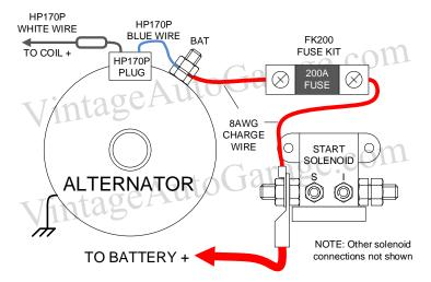
The HP170P plug and wire you installed and connected to the + side of coil tells the alternator regulator to turn on and will keep your battery charged at idle speeds this is referred as 3 wire connection. Most alternators will work as 1 wire connections and not use the plug, however the alternator will not charge at idle speeds unless RPM's are increased past the alternator internal turn on speed which is somewhere around 1400 RPM.
